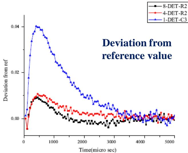
Comparison between calculated and measured value of prompt neutron decay constant.
