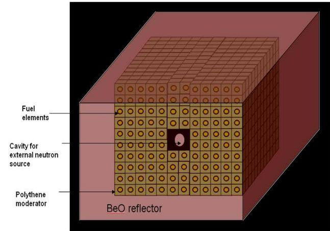
3D view of geometry used in  $K_{eff}$  calculation
