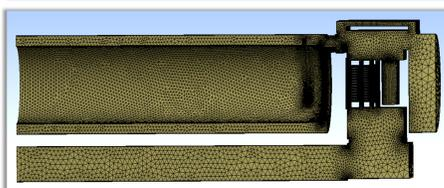
Figure 4. Cross-sectional image of full model mesh including cooling water domain.
