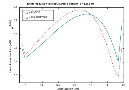
Figure 9. Linear production rate distribution at the top and bottom of RbCl Target B.
