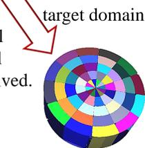
Figure 5. Simplified version of MCNP mesh for RbCl Target A with defined radial, angular, and axial planes.
