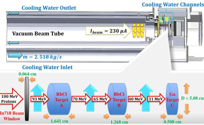
Figure 3. Cut-out of target capsules with dimensions and average incident and exiting energies crossing target faces.
