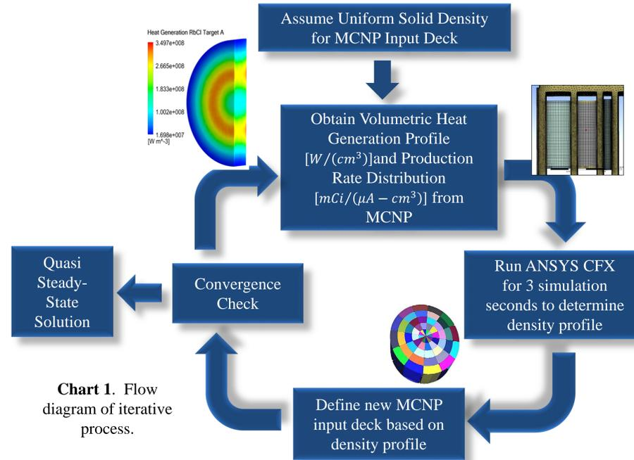
Chart 1. Flow diagram of iterative process.
