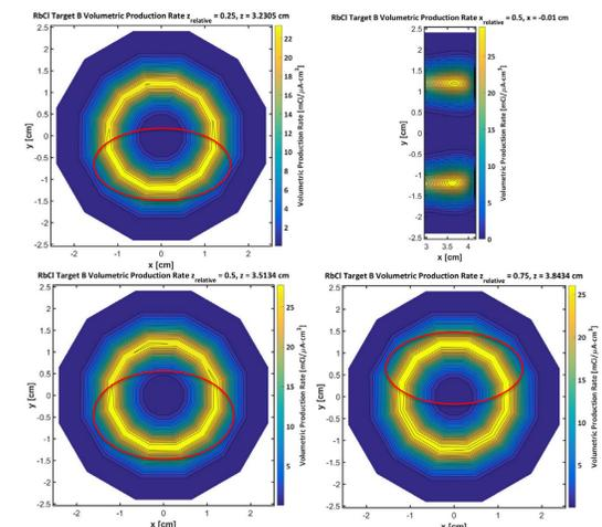
Figure 8. Volumetric production rate distributions at a YZ mid-plane in RbCl Target B and at various axial locations in XY planes with regions of highest production circled in red.
