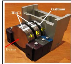
Figure 1. Routine target stack configuration at Los Alamos National Laboratory's Isotope Production Facility.
