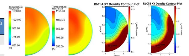
Figure 7. RbCl Targets A and B mid-plane temperature and density distribution profiles for a quasi steady-state solution.
