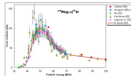
Figure 6. IAEA database cross-section data used for all yield and production rate calculations in MCNP.<sup>[5]</sup>
